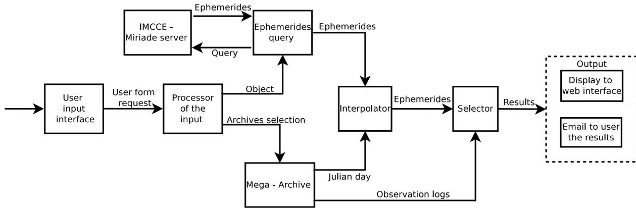
Fig. 5 The flowchart of the Mega-Precovery software.
